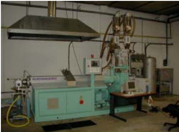
Pelletizing of coat hangers on a PME Extrusion line in the Netherland
