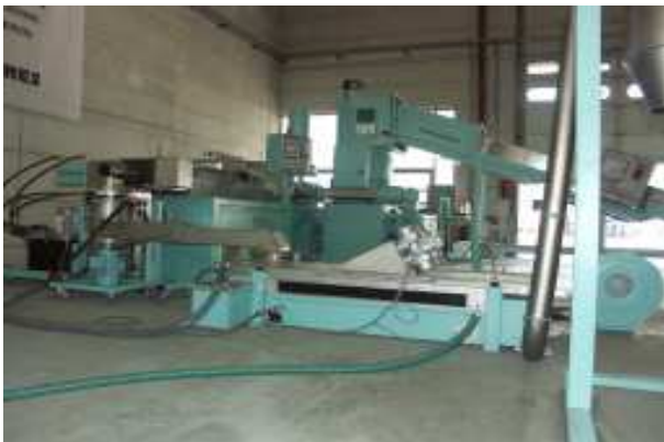
Combiline ZTE for the Processing of PP-materials to almost Virgin Quality.
