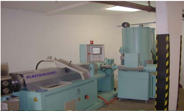
Combination Line ZTE 80 for the Reprocessing of EPS-Packaging in action.
